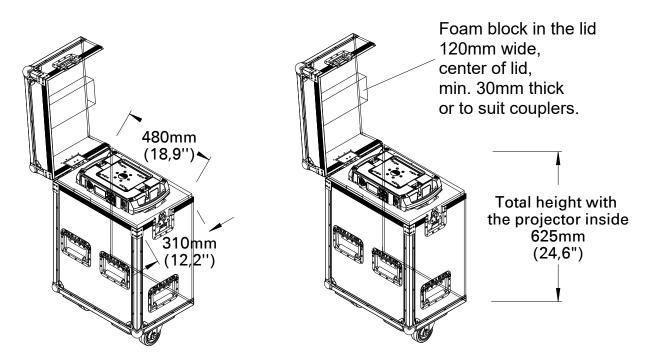
The SiP insert must be inserted into a flight case for 3x MAC Allure/Aura PXL: P/N 91515052
